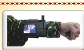
WRD-3 wrist-wear wireless A/V receiver/recorder
